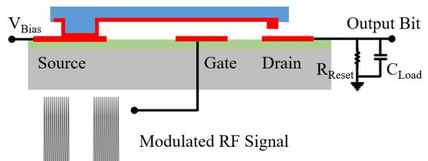
Figure 1 : Architecture of a near-zero power RF receiver
