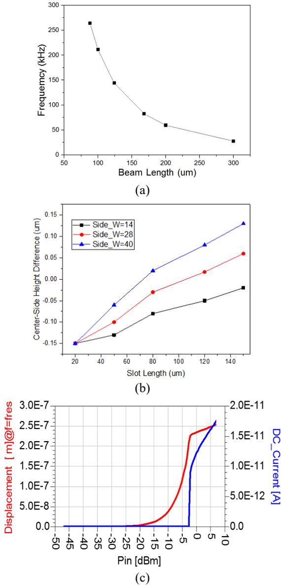
Figure 3 (a) Simulated resonant frequency of folded beam and cantilever structures as a function of beam length, (b) Simulated center beam height to side beam height difference as a function of slot length; (c) Simulated resoswitch displacement as a function of modulated input RF power.
