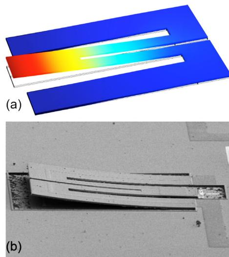
Figure 2: (a) simulation and (3D) SEM image of a  $168\mu\text{m}\times 30\mu\text{m}\times 2\mu\text{m}$  folded AlN resonant switch
