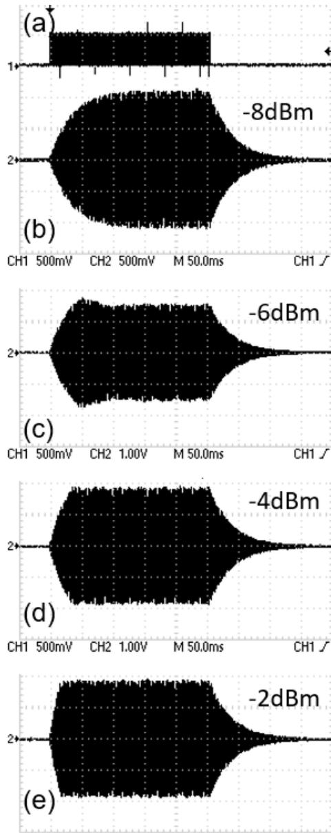
Figure 5 (a) Resoswitch input modulation signal; (b) through (e): Captured vibrometer velocity signal in response to different amplitude burst modulated signals at RF powers of (b) -8dbm, (c) -6dBm, (d) -4dBm, (e) -2dBm
