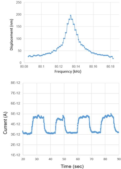
Figure 6 (a) Device resonant displacement as function of frequency; (b) resoswitch contact current at resonance when modulated RF is turned on and off at power level of -4 dBm.
